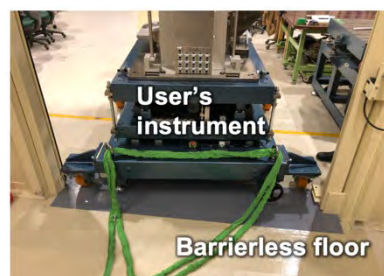
Fig. 5. Photograph of loading a user's instrument into EH2 with a barrierless floor.
